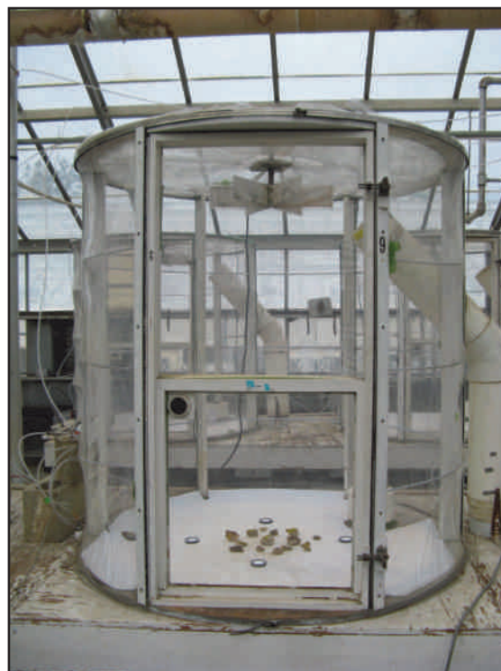
Figure 2. CSTR with lichens present at bottom of chamber. Photo by Elizabeth Hessom.
